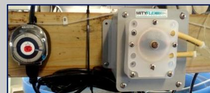
Figure 4. Peristaltic pump controlled by a cycle timer for continuous feeding microalgae to larval tanks.
